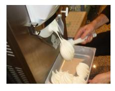
Finally you freeze the mix in a 'Batch Freezer' where the liquid mix is transformed into a complete finished Ice Cream. If extra large pieces & sauces are desired you add these as the product is drawn from the machine.
