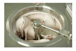
If pieces are to be added to the final product such as fruits, sauces and nuts this must be done now as the Ice Cream exits the freezer via a filler pipe (see photo). These pieces can be difficult to add unless you have a 'Fruit -Feeder' and a 'Ripple-Pump'. Each one will cost 10's of thousands, so many do it by hand with some difficulty.
