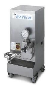
With the Industrial Method described below, during the **second** stage the mix is pumped from the Pasteuriser through a Homogeniser (a high pressure pump). This force the fat globules present to be broken down and reduced into smaller regular sized globules, to form a homogenous mix structure.
